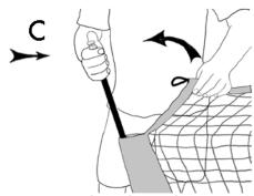
7. Grip Rod pushing direction (C) whilst pulling Orange sleeve up and looping Cord over Poll Top
