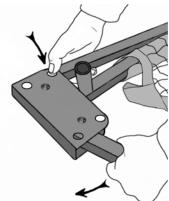
4. Depress buttons located in hinges and swing legs out
