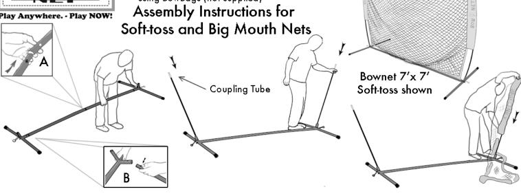
1. Join two straight Pipes together. Fig. A Then attach both end Legs. Fig. B
