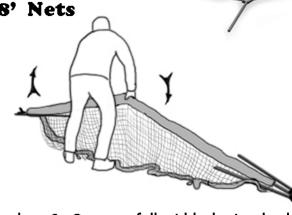
1. With center ninge on the ground. Extend frame to 6'.(1 click) for 12' net. and 9' (2 clicks) for 18' net Repeat for Other side of net
